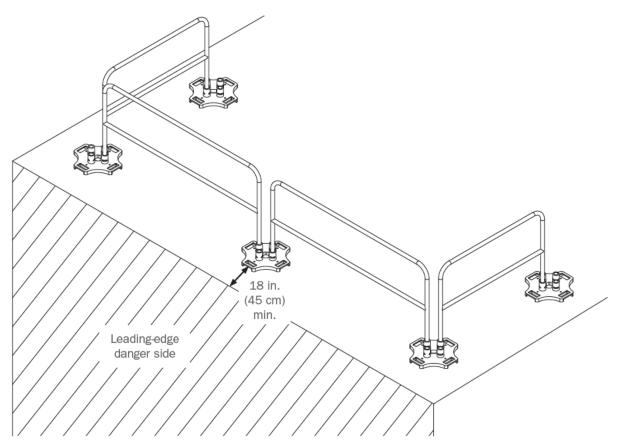
Rail sections are kept securely in place simply by inserting a lockpin through post and base.
