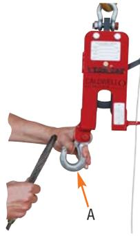
Attach catch sling to the Strip Sling Hook (A).
