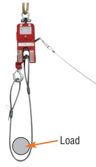
YOU ARE NOW READY TO SAFELY LIFT THE LOAD. This view shows a properly configured Rig-Release® Hook using a basket hitch.
