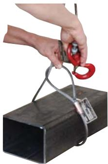
Choke the load with a separate choker sling. Attach the hook end of the catch sling to the lower eye of the choker sling.
