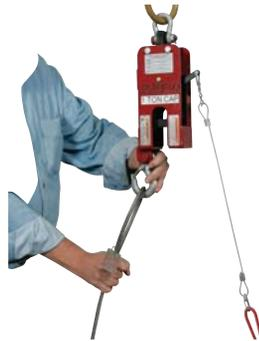
Make sure the load sling is securely in place.
