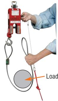
Wrap the sling around the load using a basket hitch.
